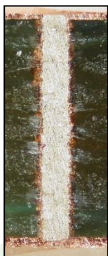
Board Thickness = 62mils Hole Diameter = 8 mils
