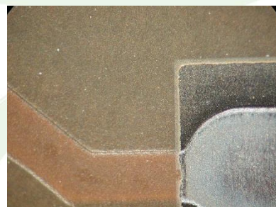
Photo 6: after 1000 hours over FR4 laminate
