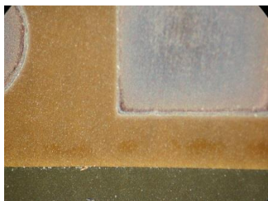
Photo 1: after 250 hours over copper
