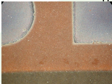
Photo 3: after 500 hours over copper
