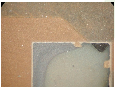
Photo 7: after 2000 hours over copper
