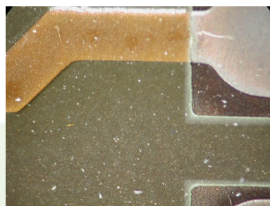
Photo 2: after 250 hours over FR4 laminate
