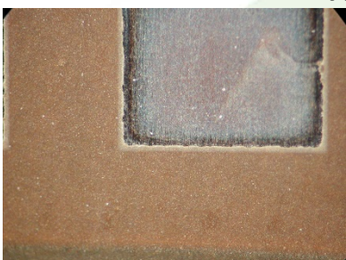
Photo 5: after 1000 hours over copper
