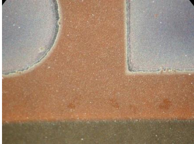
Photo 5: after 1000 hours over copper
