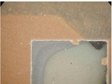
Photo 7: after 2000 hours over copper
