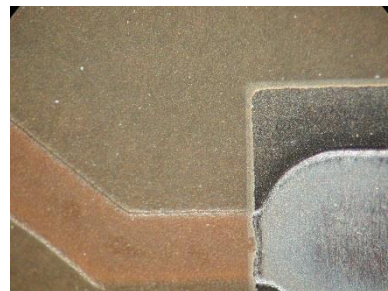
Photo 6: after 1000 hours over FR4 laminate
