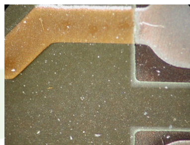
Photo 2: after 250 hours over FR4 laminate
