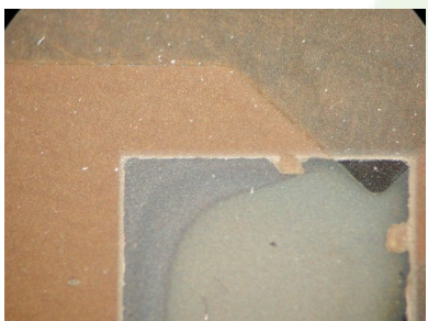
Photo 7: after 2000 hours over copper
