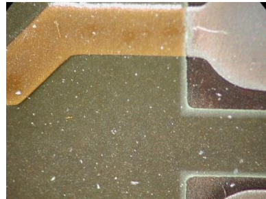
Photo 2: after 250 hours over FR4 laminate
