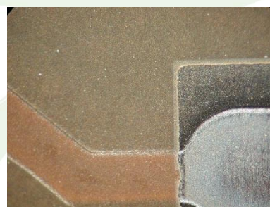
Photo 6: after 1000 hours over FR4 laminate
