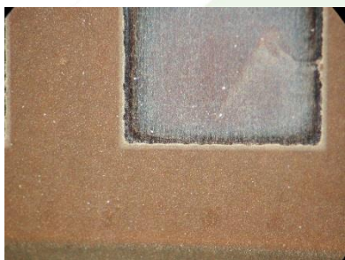
Photo 5: after 1000 hours over copper
