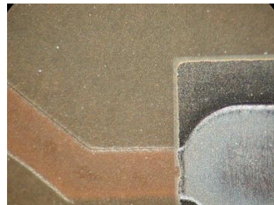
Photo 6: after 1000 hours over FR4 laminate
