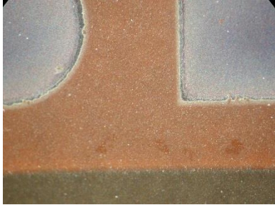
Photo 3: after 500 hours over copper
