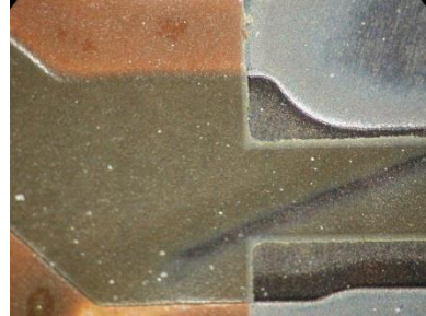
Photo 4: after 500 hours over FR4 laminate
