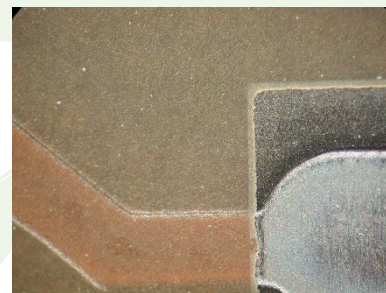
Photo 6: after 1000 hours over FR4 laminate
