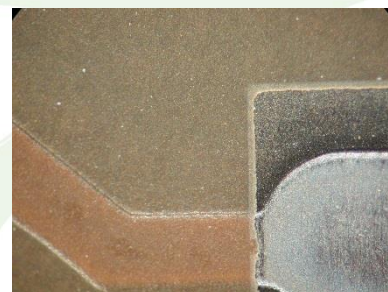
Photo 6: after 1000 hours over FR4 laminate
