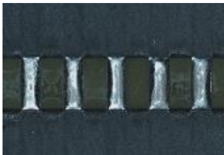
Base material: FELIOS R-F775 (PI: 25 μm, Cu: 18 μm, Panasonic ) Fig. Surface observation after solder heat resistance (288deg.C 10 sec. × 3 times).
