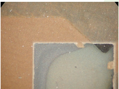
Photo 7: after 2000 hours over copper
