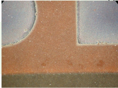
Photo 3: after 500 hours over copper
